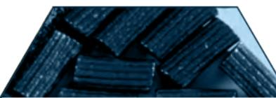
Anti tank gun propellant
